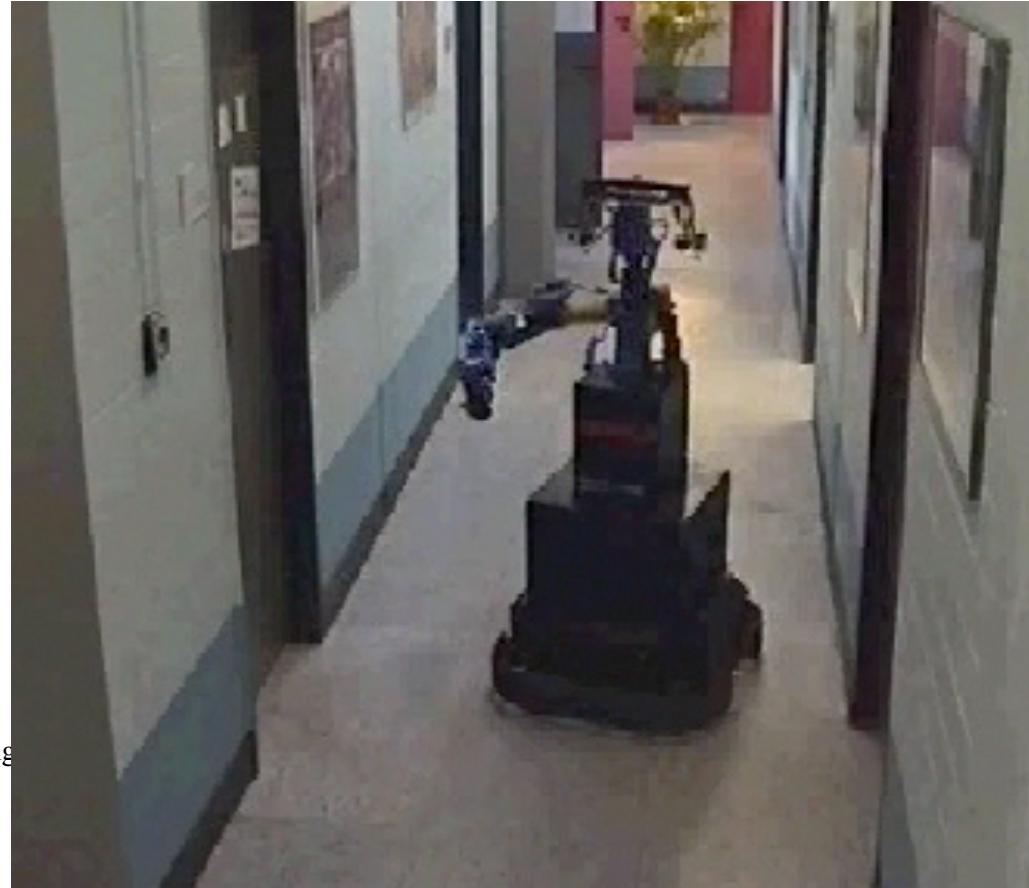
.28. Dexterous arm on mobile base, opening door (left), robot passing through doorway (right)
