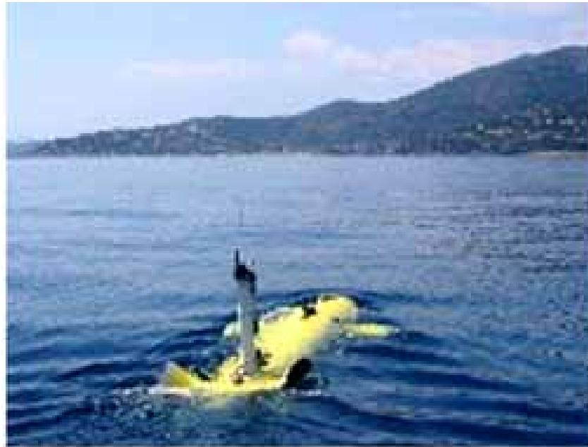
Figure 2.2. IFREMER ASTER autonomous underwater vehicle.
