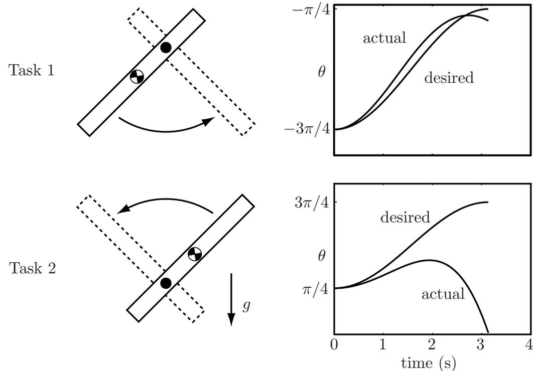
**Figure 11.17:** Results of feedforward control with an incorrect model:  $\tilde{r} = 0.08$  m, but  $r = 0.1$  m. The desired trajectory in Task 1 is  $\theta_d(t) = -\pi/2 - (\pi/4)\cos(t)$  for  $0 \leq t \leq \pi$ . The desired trajectory for Task 2 is  $\theta_d(t) = \pi/2 - (\pi/4)\cos(t)$ ,  $0 \leq t \leq \pi$ .
