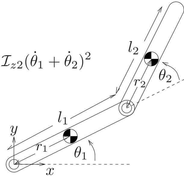
$$\begin{bmatrix} \alpha + 2\beta c_2 & \delta + \beta c_2 \\ \delta + \beta c_2 & \delta \end{bmatrix} \begin{bmatrix} \ddot{\theta}_1 \\ \ddot{\theta}_2 \end{bmatrix} + \begin{bmatrix} -\beta s_2 \dot{\theta}_2 & -\beta s_2 (\dot{\theta}_1 + \dot{\theta}_2) \\ \beta s_2 \dot{\theta}_1 & 0 \end{bmatrix} \begin{bmatrix} \dot{\theta}_1 \\ \dot{\theta}_2 \end{bmatrix} = \begin{bmatrix} \tau_1 \\ \tau_2 \end{bmatrix}$$
