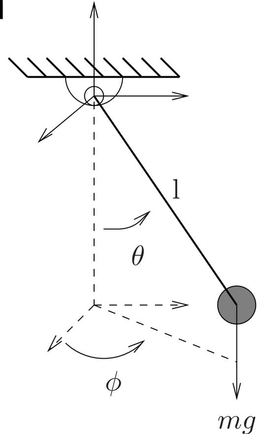
position relative to base  $r(\theta, \phi) = \begin{bmatrix} l \sin \theta \cos \phi \\ l \sin \theta \sin \phi \\ -l \cos \theta \end{bmatrix}$
