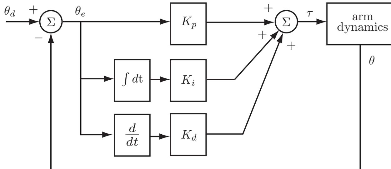
Figure 11.12: Block diagram of a PID controller.
