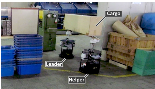
Fig. 1 The team of autonomous mobile robots transporting a long box as cargo/payload. Here, the validation scenario is a factory floor
