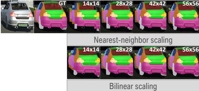
Fig. 4: Visual comparison of the resulting multi-class masks for the same detection using the nearest-neighbor or bilinear scaling method. The different kernel sizes imply different underlying network weights.
