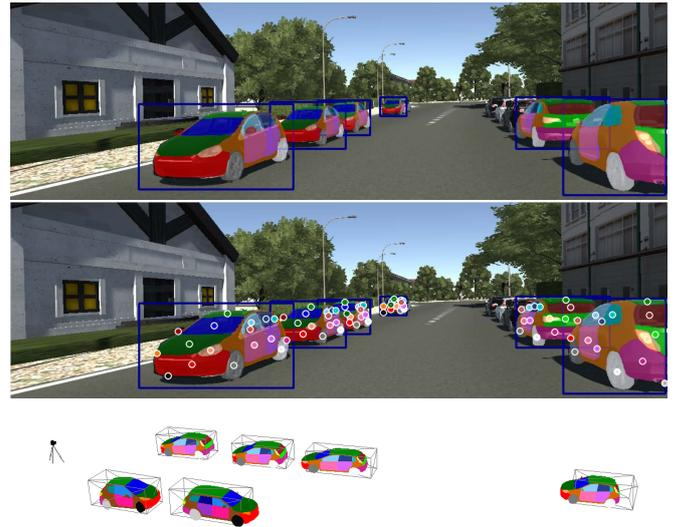
Fig. 1: Exemplary result from the presented 6DoF pose estimation pipeline. *Top*: Prediction of the multi-class Mask-RCNN on the Virtual KITTI dataset [1]. Our vehicle detector outputs part-level segmentation masks. *Middle*: For each detection, part correspondences (colored points) are generated from the segmentation mask and passed to a PnP-solver. *Bottom*: Resulting 3D Visualization of the 6DoF vehicle poses, black boxes represent the ground truth.
