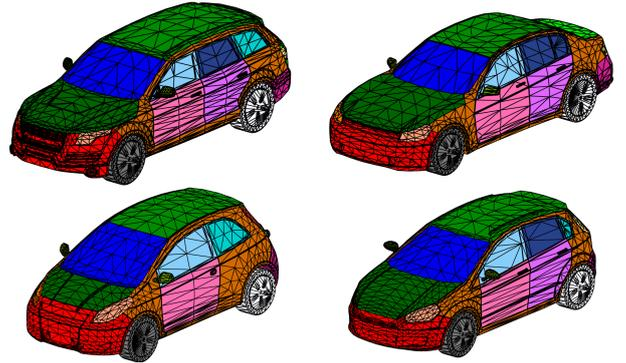
Fig. 2: Visualization of the multi-class vehicle representation annotated on four CAD models.
