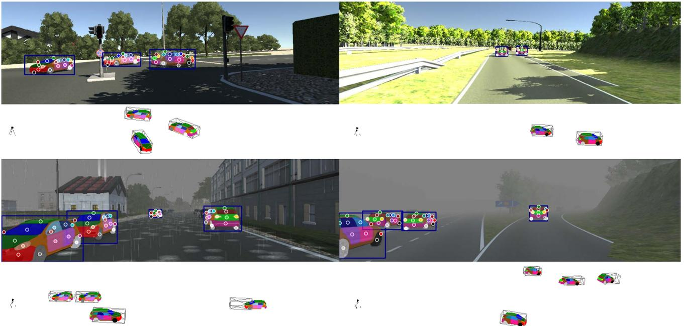
Fig. 5: Several example frames from the evaluation on the Virtual KITTI dataset [1]. The upper half of the example shows the processed frame with bounding box vehicle detections, mask predictions and calculated center points (colored dots). The lower half shows the 3D visualization of the scene with the predicted models for detections and wireframe bounding boxes for ground truth.
