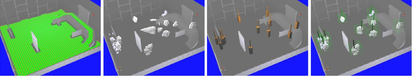
Fig. 2. From left to right: Walkable area marked in green with red grid points. Active voxels from the SFS reconstruction. SDD detections. Detections fused with volumes and bounding boxes.
