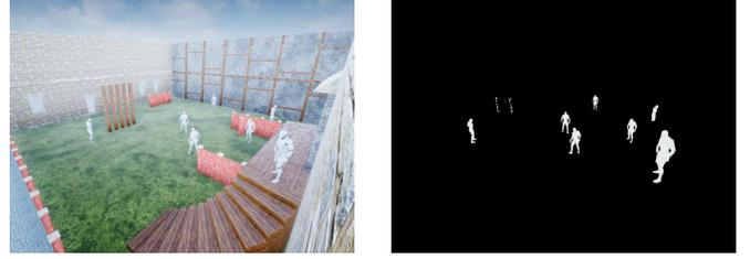
Fig. 3. Example of virtual experiment input from the *occluded* scenario. Both images were generated with Unreal Engine 4 *Left*: Virtual camera image of sample test environment. *Right*: Corresponding binary segmentation image.
