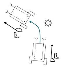
The vehicle's change in angle depends on its current sensor input
