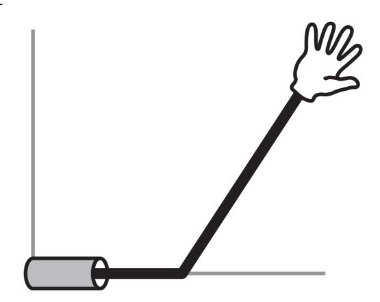
(the first joint is the prismatic 'slider' joint)
