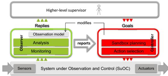
Fig. 1. Conceptual view of an individual Sissy system.
