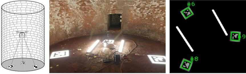
Fig. 7: The setup and exemplary recording from the down-facing wide-angle camera. LED panels with printed AprilTags are placed on the ground in an arbitrary arrangement (left and center). The robot detects these markers (right) and derives an absolute measure of orientation.
