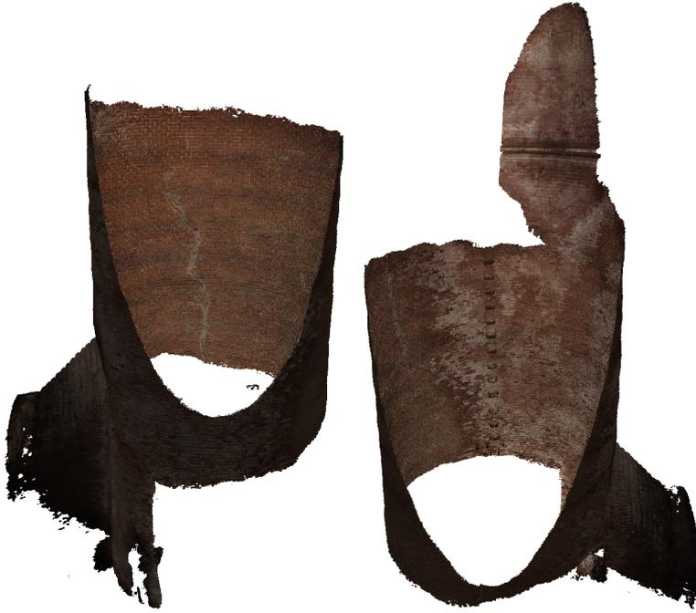
Fig. 17: 3D reconstruction of the Zollverein chimney. In addition to the spiral coverage of the chimney, the MAV covered a part from the bottom to the begin of the pattern during start, and a higher part of the chimney with a straight ascending flight before landing.
