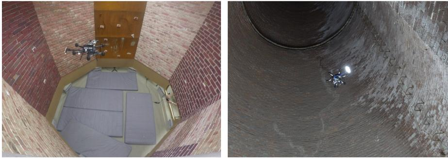
Fig. 2: Autonomous chimney inspection. Our lightweight chimney inspection MAV navigates autonomously assisted by real-time 6D laser localization and fast visual odometry. A spiraling scan pattern facilitates good and efficient coverage for camera-based surface reconstruction of the chimney walls. Our MAV is evaluated in a narrow chimney mock-up (left) and a decommissioned industrial chimney (right).
