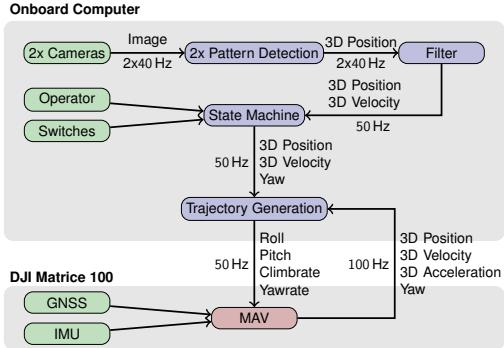
Fig. 3. Structure of our method. Green boxes represent external inputs like sensors, blue boxes represent software modules, and the red box indicates the MAV hardware. All software components use ROS as middleware. Position, Velocity, Acceleration and Yaw are allocentric.
