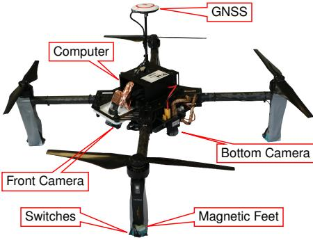
Fig. 2. Design of our MAV equipped with two cameras, magnetic feet, and a lightweight but fast onboard PC (shielding removed for better view).
