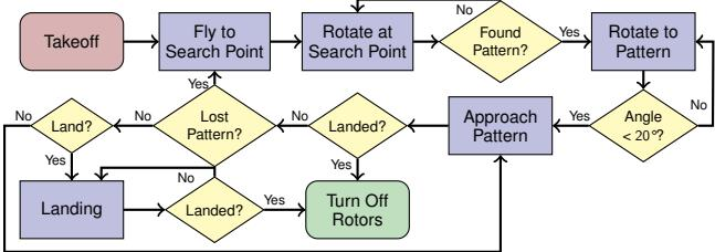
Fig. 6. The flowchart of our state machine. Besides the basic behavioral control, it features strategies to recover from failed landing approaches.
