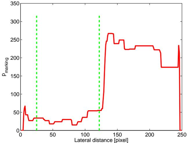
Fig. 4: The function  $p$  computed on the image in Fig. 3. The two markings indicate the minimal distance of the parking lots and the position the signal significantly changes, respectively. The first is needed to estimate the noise of the signal, the latter provides the estimated parking lot distance.
