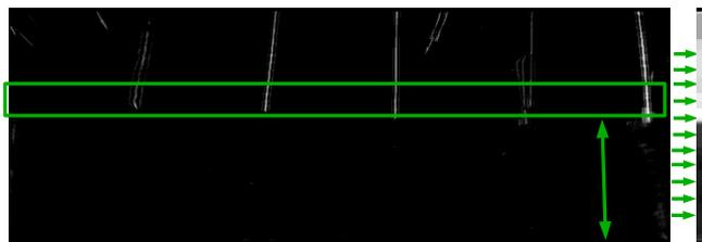
Fig. 3: The symmetry image provides a likelihood for the presence of bright vertically oriented structures of a given size (here:  $\approx 10\text{cm}$ ). The lateral distance to the parking lot (green arrow) can be determined by means of the function  $p$  that transforms each scan-line into a likelihood of a parking lot pattern being present (*cf.* Sec.III-B). The green rectangle shows the area that is subsequently regarded for computing the offset and parking lot width (*cf.* Sec.III-C).
