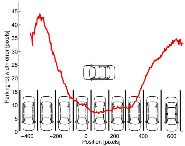
(b) The error in parking lot width estimation w. r. t. the relative vehicle position. The widths of parking lots close to the car can be pinpointed with an error of 10.4 pixels ( $\approx 0.21$  meters)
