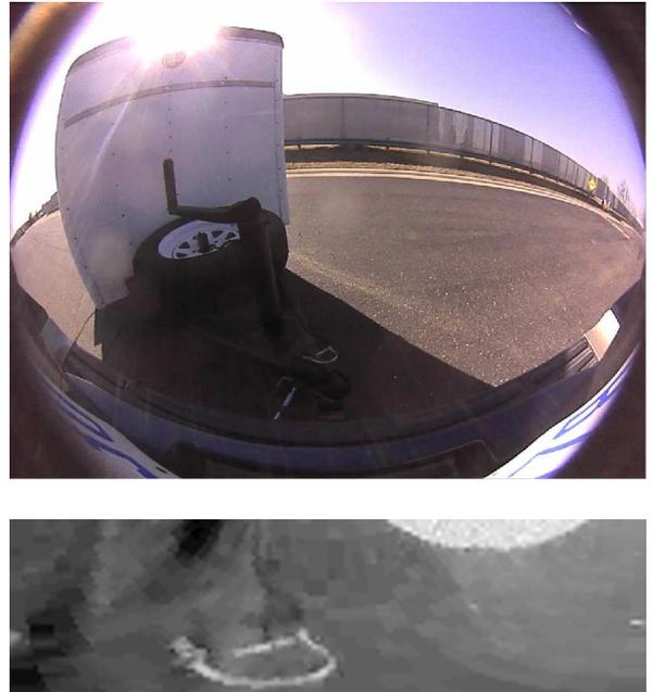
Fig. 1: An example image for articulation estimation. The trailer’s shadow creates a symmetric structure (upper right corner) in the transformed image (logarithm shown) that may be confused with the drawbar axis, as it creates strong edges whereas the drawbar itself is hard to detect. This situation confirms the need for a relative brightness measure and a careful selection of all symmetry maxima.
