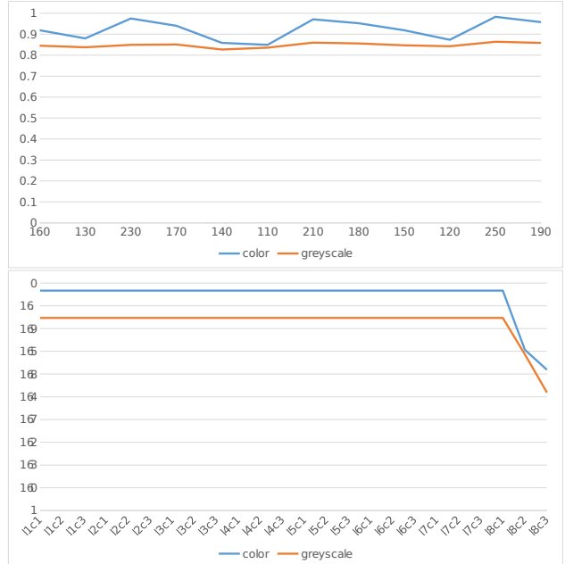
Fig. 3. Recognition rates on ALOI depending on illumination direction (top) and illumination type (bottom). The cues for the color evaluation were HHI, LBP, SHI, and BHI), for greyscale PCC, CHI, LBP and BHI.
