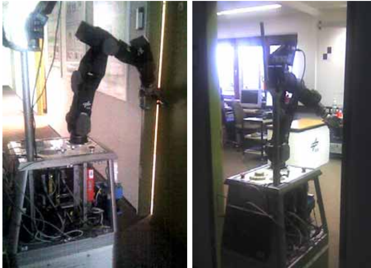
Figure C.28. Dexterous arm on mobile base, opening door (left), robot passing through doorway (right).
