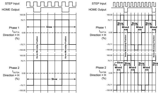
Figure 4. This image shows sequences of the electric currents driven through the coils of the stepper motors (phase 1 and phase 2) by the microstepping controller A3979. On the left, the *full-step* mode is shown; on the right the *half-step* mode. The frequency of the incoming step impulses regulates the motor speed; the more intermediate steps are made, the smoother the motor is running. (Source: [2])
