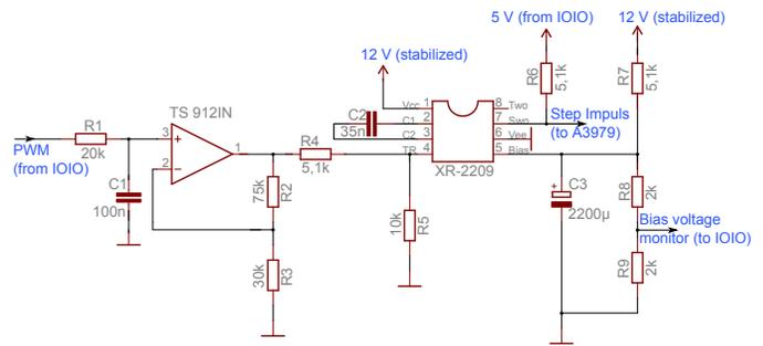
Figure 6. This image shows the circuitry for generating an impulse sequence with variable frequency via a PWM signal with fixed frequency.
