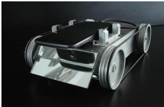
Figure 1. A view of the robot with mounted smartphone and the mirrors enabling stereo vision.
