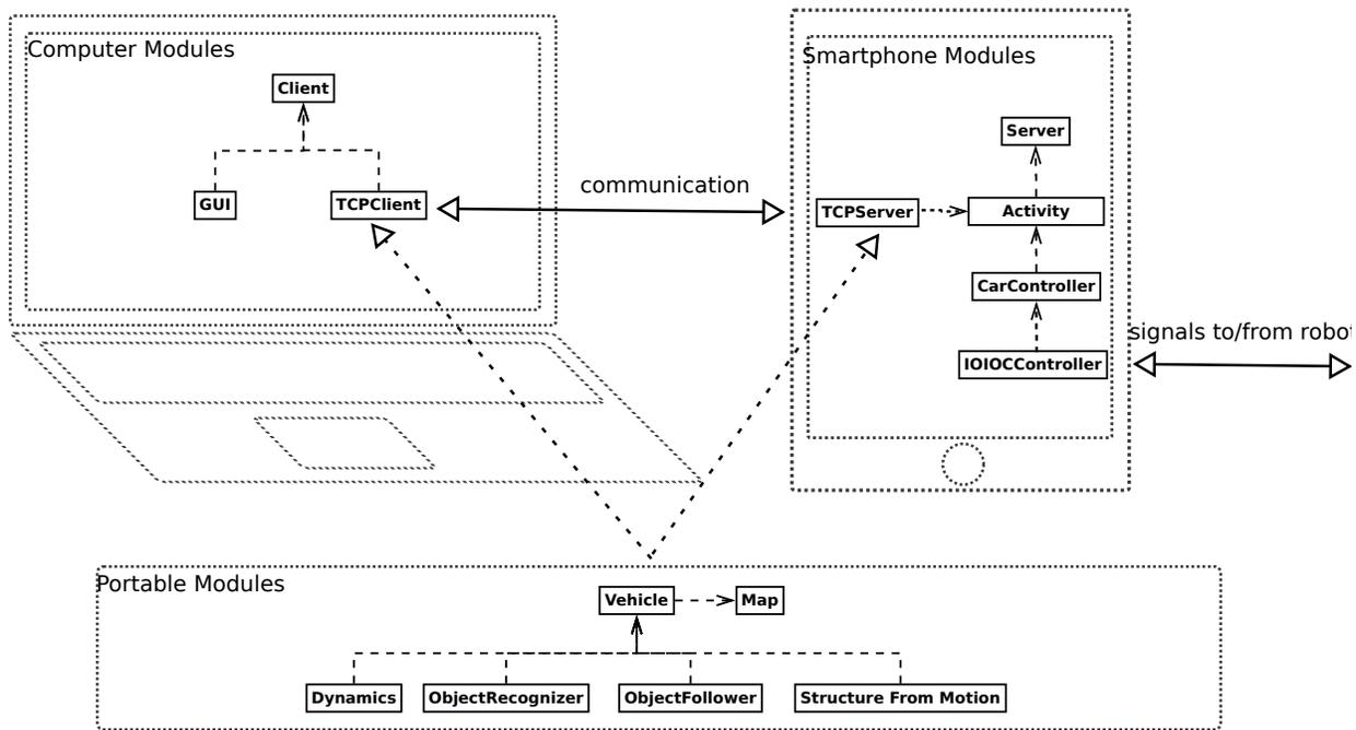
Figure 8. This figure shows the main software modules. Hardware controllers run directly on the smartphone, for interaction a GUI on the laptop is used. Portable modules can run on the smartphone but may also be moved to the laptop if more computational resources are required.
