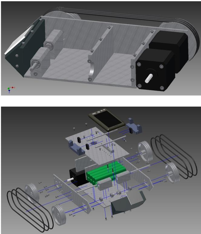
Figure 2. An internal view of the robot chassis and an exploded view of the whole robot without the stereo vision device
