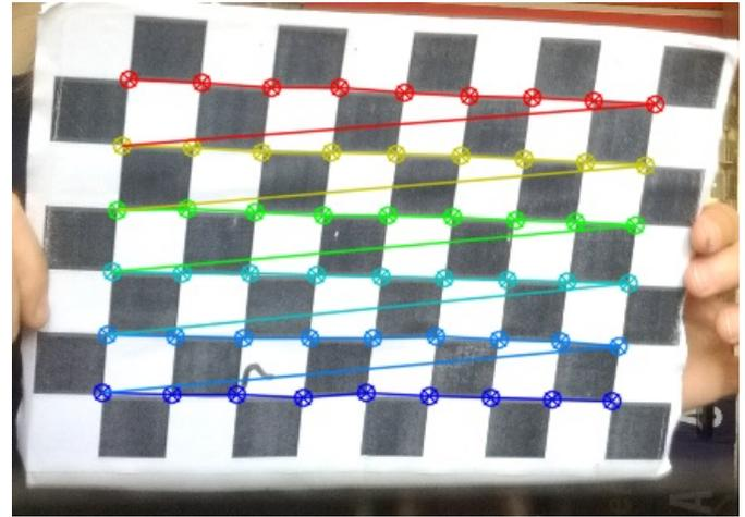
Figure 12. The calibration chessboard.
