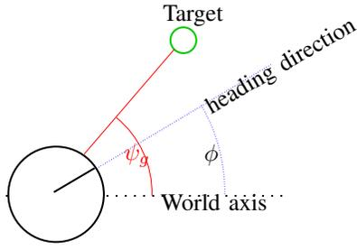
Figure 13. The robot, its heading direction and the angles.
