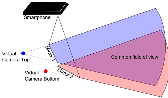
Figure 7. Schematic illustration of the optical system for Stereo Vision with a single camera; the angle and offset between the two mirrors create two virtual camera positions; the distance between these virtual camera positions is fixed, so it can be used for three-dimensional reconstruction of the environment.
