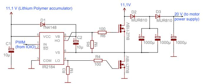
Figure 5. Circuit diagram of the charge pump (circuitry based on [3])
