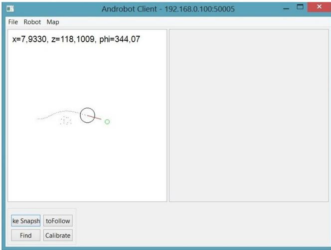
Figure 9. This is the main window of the Client application that is used to show the path and map data of the robot. It is also possible to manually send control commands to the robot to let it move.
