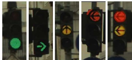
Fig. 1. Examples of the different types of traffic lights we aim to distinguish. All four different phases and possible pictograms are shown.
