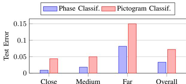
Fig. 12. The error on the test dataset with respect to the distance between camera and traffic light. This distance has direct implications on the size of the observed lights. “Close” represents lights with a diameter of more than 14 pixels. “Far” represents lights with a diameters of 8 pixels or fewer. Lights with a diameter between 8 and 14 fall into the category “Medium”.
