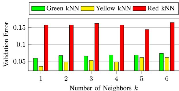
Fig. 7. The error of each kNN classifiers on the validation set for different values of  $k \in [1, 6]$ . Minimal values are found at  $k = 1$  for green and yellow kNNs and at  $k = 5$  for the red kNN. For better readability we omitted values between 7 and 10 – here the performance on the validation set is worse.
