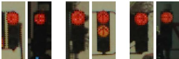
Fig. 13. Examples of pictograms on red lights. It can be seen, that even on lights of medium size the arrow is very blurry and hard to recognize. The two left images show arrows to the left, the two middle images to the top, and the two images on the right to the right.
