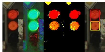
Fig. 3. In this example the color definitions for red and yellow overlap (as detailed in Sec. V). This is indicated by orange color in the segmentation images. The shapes of  $R_r$  and  $R_y$  are adapted so that they do not intersect.
