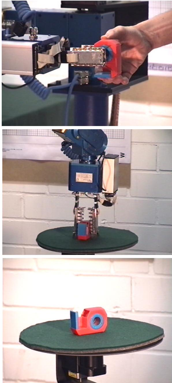
**Fig. 4.** Learning the representation of a new object. The object is placed into the gripper such that a stable grip is known (top). The robot puts the object onto a turntable (middle) and images of the various views are recorded without interference from the gripper (bottom).
