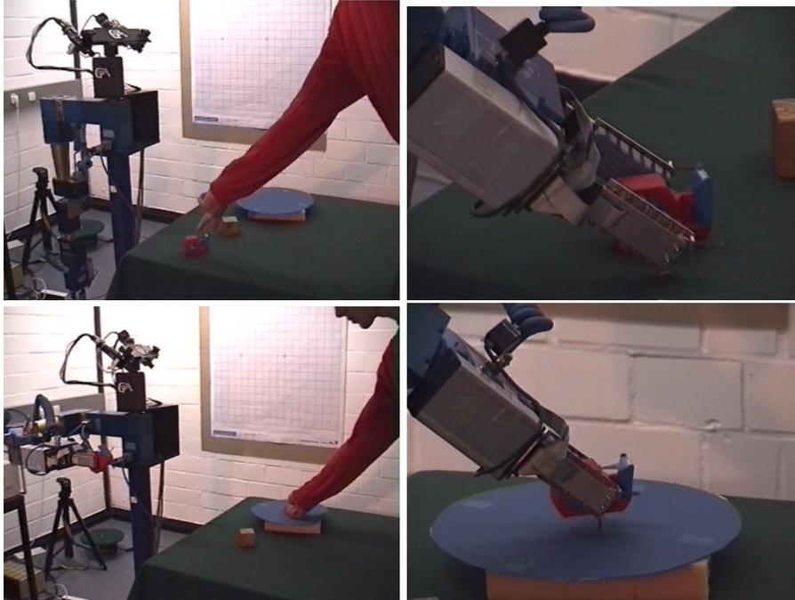
**Fig. 3.** Pick- and place behavior. The user points at one of the objects with a hand gesture (top left). The hand gesture is recognized and the closest object is picked up at the angle indicated by the gesture (top right). The robot waits for a new gesture (bottom left) and places the object at the indicated position (bottom right).
