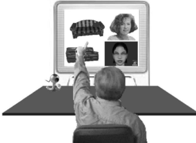
**Fig. 1.** Possible application of multimodal man-machine-communication in a *virtual shop* scenario: the user communicates with an artificial personal assistant on his tv-set (here in the lower right corner of the screen) by means of speech, gaze, pointing- and head-gestures using uncalibrated cheap devices like webcam and microphone. A combination with a video-conferencing system for the simultaneous communication with human partners (upper right) is planned.
