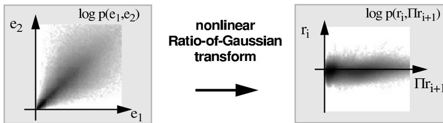
Fig. 6. The joint statistics of the response  $r_i$  of a ROG operator and of the set of remaining channels  $\Pi r_{i+1}$  are much closer to statistical independence (cf. Fig. 2) (note that in analogy to eq. (1)  $\Pi r_{i+1} = \sum d_{i+1} = g_{i+1}$ , i.e it is also equivalent to the local mean)
