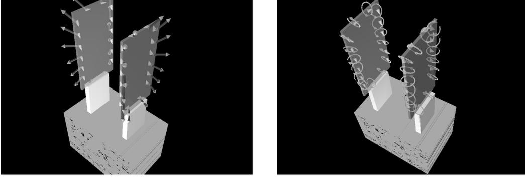
Fig. 9. The translational (left) and rotational (right) vector fields of the inner hair sensors. The translational one is radial in order to center the gripper around an object, and the rotational one is circular in order to orient the gripper parallel to the object surface.
