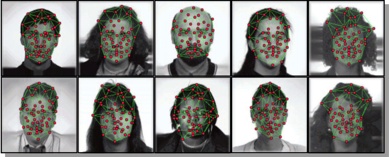
Figure 1. Bunchgraph Matching [27]. This figure shows a variety of images with the graphs corresponding to a fixed bunch graph overlaid. It can be seen that the positions of many landmarks are estimated well. These graphs can also be used to extend the original bunch graph.
