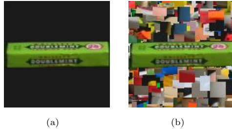
Fig. 15. Input Images of a Single Object — The figure shows an object from the COIL-100 database [21] as (a) segmented and (b) unsegmented image. Since the images of that database are perfectly segmented, the unsegmented images have been manually created by pasting the object contained in the segmented image into a cluttered background consisting of arbitrarily chosen image patches of random size derived from the other test images of the current testing set. This is the worst background for feature-based systems.
