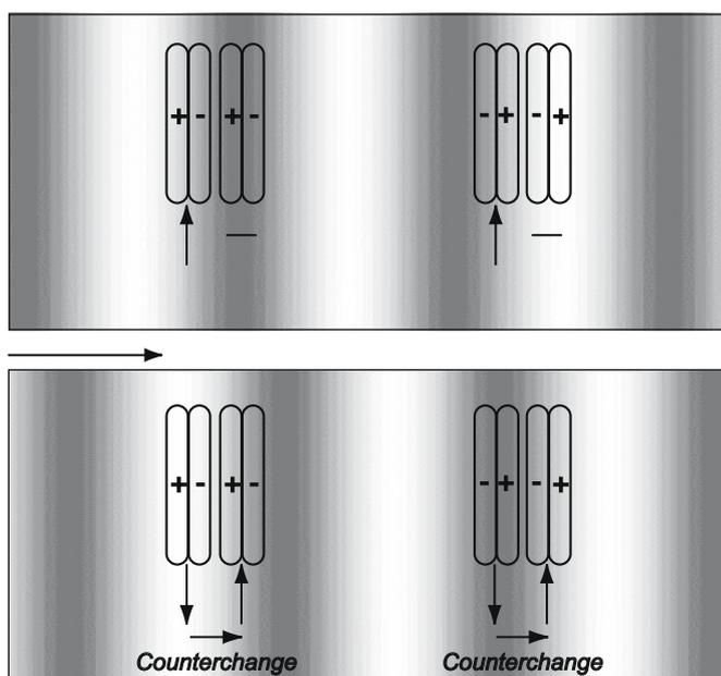
**Fig. 14.** Illustration of how the perception of motion for a drifting sine grating can be based on the detection of counterchange when the inputs to the biphasic subunits of the counterchange motion detector come from spatial filters with one excitatory and one inhibitory lobe (i.e., edge detectors). The optimal input for counterchange detection comes from pairs of filters that are 90° out of phase with respect to the spatial frequency of the sine grating.
