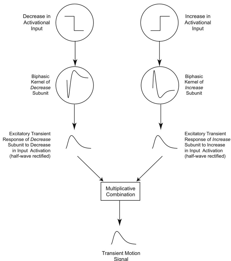
Fig. 2. Description of the counterchange motion detection mechanism.
