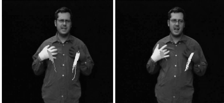
Fig. 15.8. The trajectories and static hand gestures of the signs “excited_interested” (left) and “live” (right) are very similar. Therefore, the shorter sign live dominates the recognition of the excited_interested performance. The integration of non-manual observation like a grammar or facial expression should help to differentiate between similar signs.
