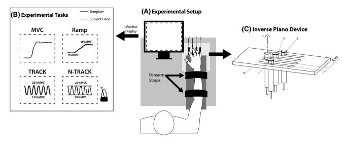
Fig. 1 a A schematic of the experimental setup showing the subject's position and the sensor arrangement; b illustration of the feedback given to the subject on the monitor display. Signals for the maximum voluntary contraction (MVC), ramp force production, and cyclic force production with (TRACK) and without (N-TRACK) template are illustrated. A metronome paced the N-TRACK task; c schematic
