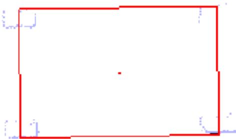
Fig. 5. A detected hypothesis (red rectangle) by the RANSAC algorithm and corresponding LIDAR measurements (blue dots).
