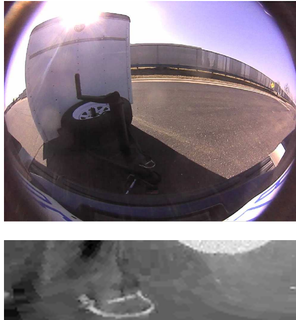
Fig. 1: An example image for articulation estimation. The trailer’s shadow creates a symmetric structure (upper right corner) in the transformed image (logarithm shown) that may be confused with the drawbar axis, as it creates strong edges whereas the drawbar itself is hard to detect. This situation confirms the need for a relative brightness measure and a careful selection of all symmetry maxima.
