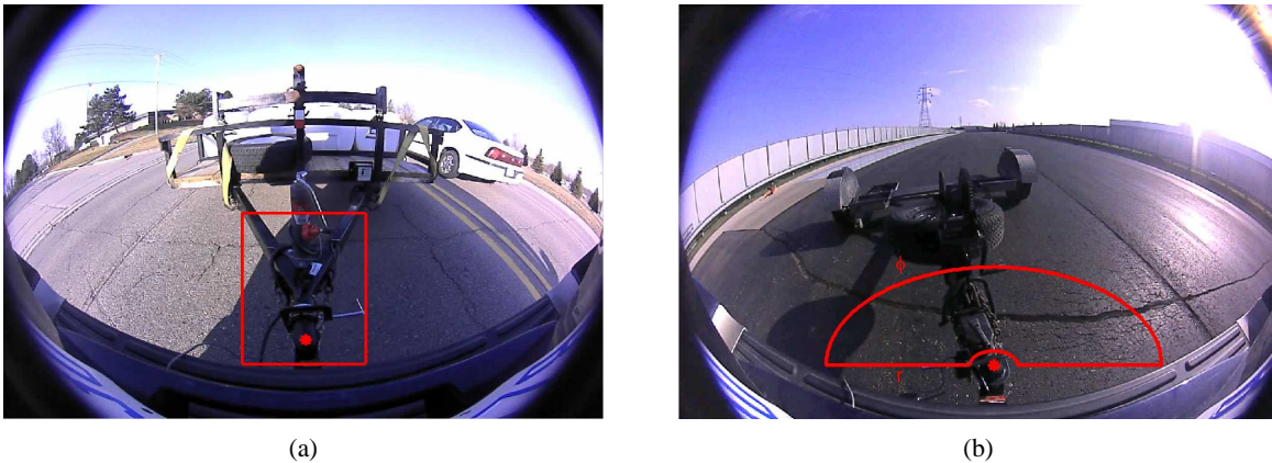
Fig. 2: 2a The surrounding of the hitch that is taken into account for detecting the presence of a trailer. 2b The definition of the polar coordinate system to transform the area around the hitch for later symmetry analysis.
